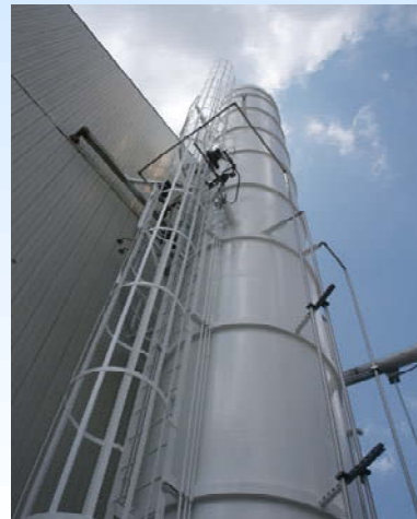
ONE OF SEVERAL ARENCIBIA “COLD BOX” CONDENSERS IN OPERATION
